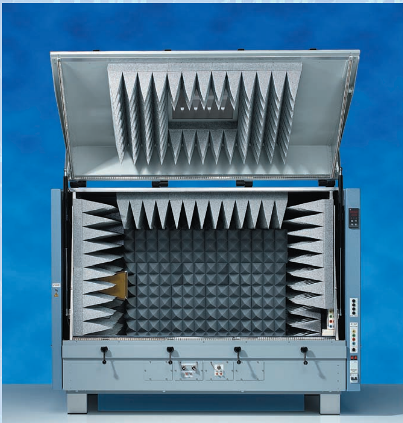
FIG 3 A horn antenna is mounted on the left inside wall of M-LINE; it serves for radiating signals into the cell and for receiving emissions from the EUT
