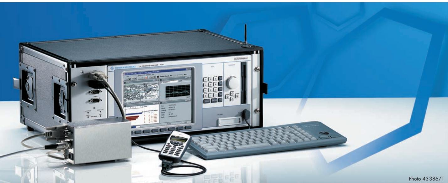
FIG 1 Interference measurement system ROGER – compact and lightweight for mobile use
